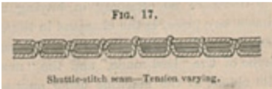
FIG. 17. Shuttle-stitch seam-tension varying.
